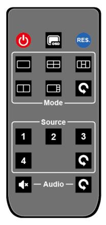
Press this button to setting standby mode, press this button again to power on the unit.
