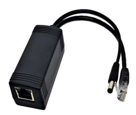
ATZ POE-SP3202-at, a cost-effective and highly reliable remote PoE PD device based on standard IEEE802.3at, transmitting power and data through a splitter cable. It provides power and data to devices without PoE function when connecting with a PoE Switch or PSE Injector. The output voltage is 12V, and equipped with PoE power supply device, it could effectively expand the scale of Security Surveillance & Wireless Network without the limitation of power line layout.
